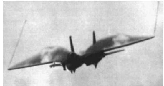
Figure 18. Condensation showing the distribution of lift along a wing.
