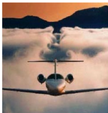
Figure 7. Downwash and wing vortices in the fog.
